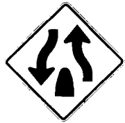
DIVIDED HIGHWAY ENDS
